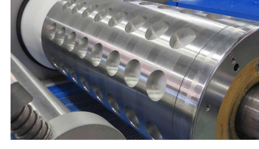
For test batches or development of new products, the New Product Development drum can be used. Its interchangeable segments allow you to experiment with different product shapes and sizes.
