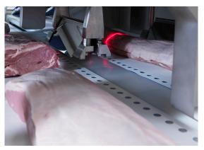
Product scanned by vision system for high-accuracy portioning.
