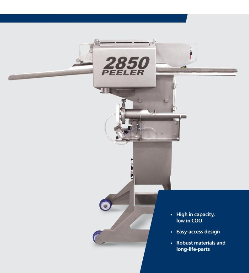
The Townsend 2850 Pepperoni Peeler accurately removes the inedible dried casing from your pepperoni without damaging the pepperoni itself. The high capacity peeler can handle a wide variety of products, with a caliber range from 35 to 50 mm and a length range from 250 to 1500 mm.
