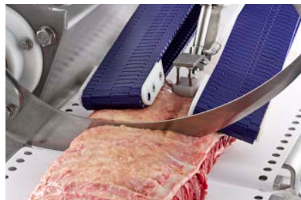
Product supported by product holder & back hold fork during cutting
