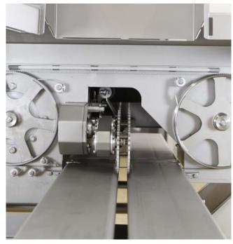
Open cover showing horizontal band saw
